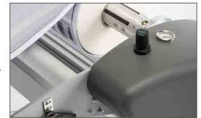
Pneumatic brake for adjusting the media tension
