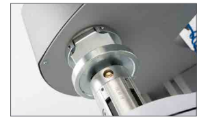
Ease of loading heavy rolls thanks to the air expansion shaft
