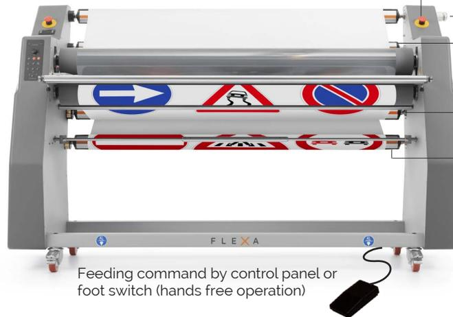
Rewinding shaft with clutch
