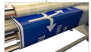
Rear rewinding shaft with clutch and shedding bar (optional)
