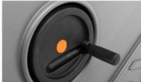
Manual lifting of the upper roller with the hand-wheel (motorized lifting optional)
