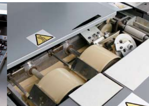
Glue drums with automatic side gluing and glue cut off control
