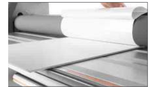
Aluminium extra-deep feed table ideal for mounting the graphic on the board
