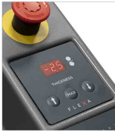
Motorized lifting of the upper roller (optional)
