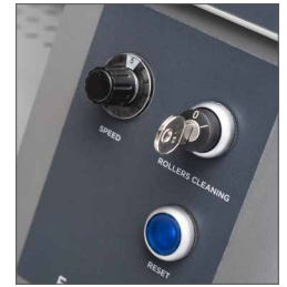
Electronic working speed adjustment by potentiometer
