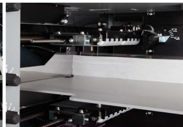
Accurate and reliable A.M.S.+ Suction Feed System
