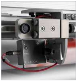
Optical sensor for vertical alignment
