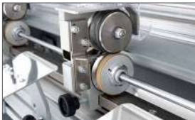
Lengthwise shear cutters (twin cutters optional)
